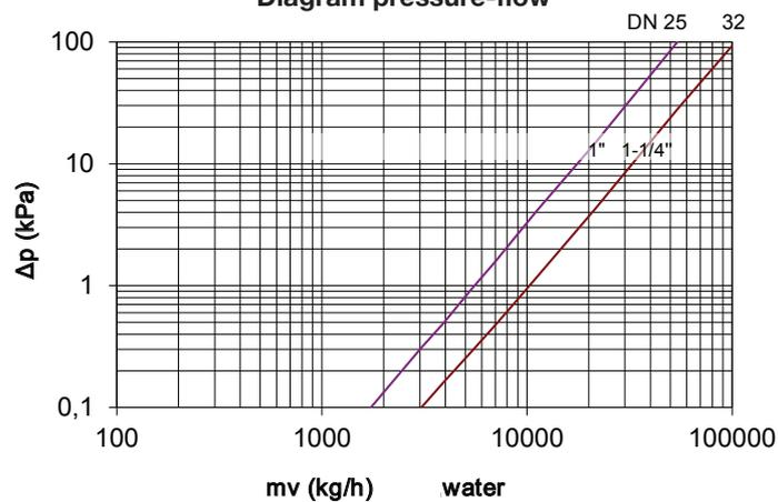
**Kv:** Outflow characteristic (m<sup>3</sup>/h) - is the flow of water at temperature 15.5°C, a pressure drop of 1 bar (100 kPa) and a fully open valve.
