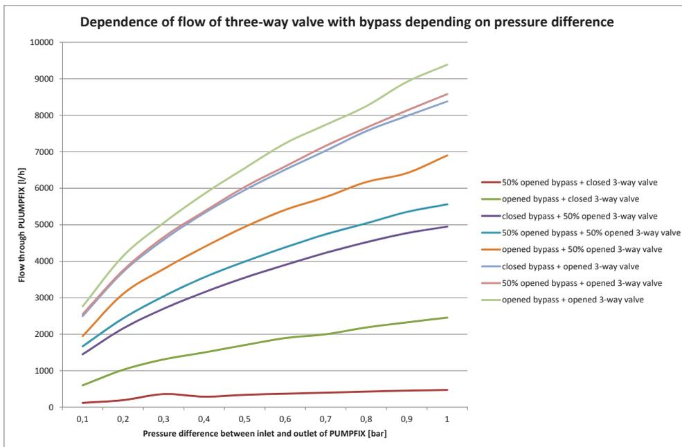
**Characteristic curves of three-way valve (closed bypass)**
