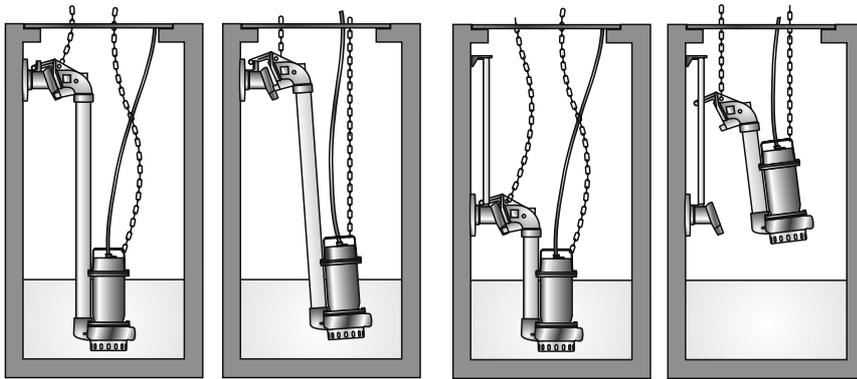
In installations in which the DAC-E needs to be fastened far from the well cover, two guide pipes (3/4") may be used, which are helpful for accompanying the electric pump until it is perfectly coupled.
