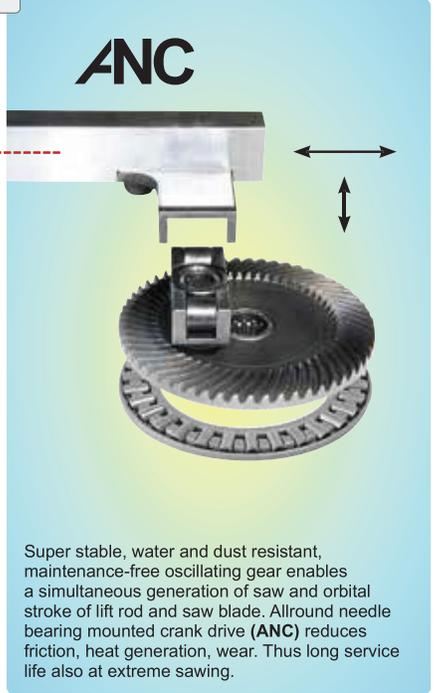
Super stable, water and dust resistant, maintenance-free oscillating gear enables a simultaneous generation of saw and orbital stroke of lift rod and saw blade. Allround needle bearing mounted crank drive (ANC) reduces friction, heat generation, wear. Thus long service life also at extreme sawing.
