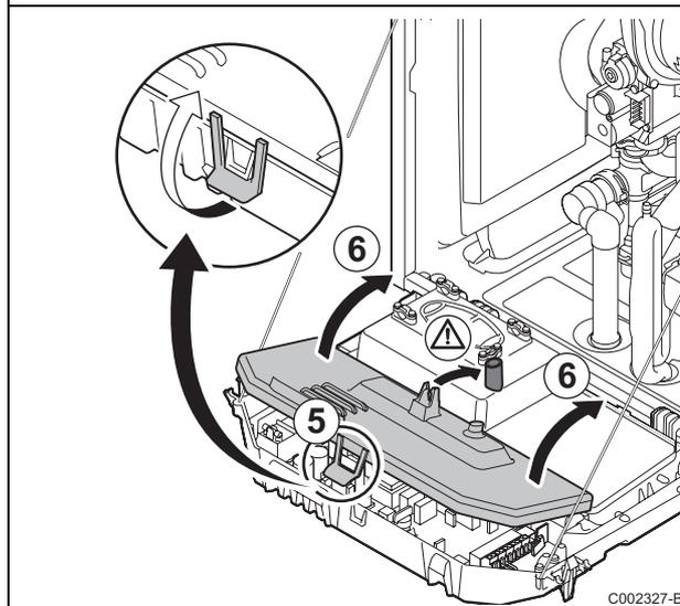
5. Lift the clip located in front of the control panel
