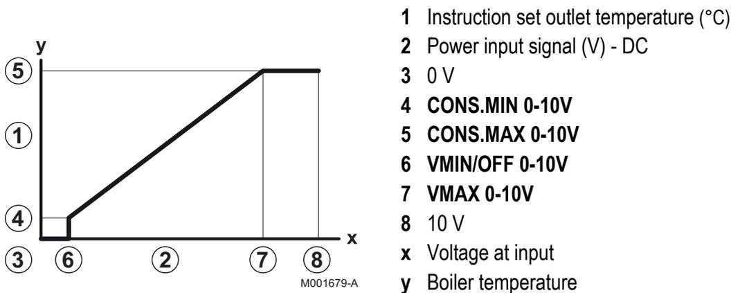
If the input voltage is less than **VMIN/OFF 0-10V**, the boiler is off.
