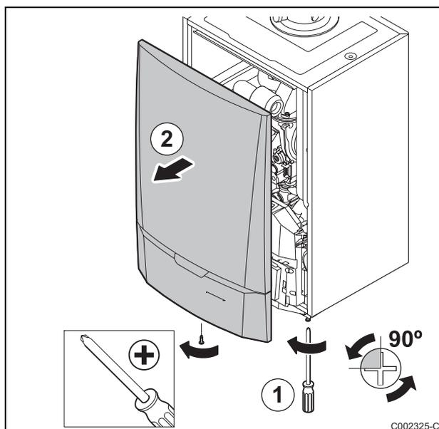
1. Unscrew the 2 screws under the front panel by a quarter turn
