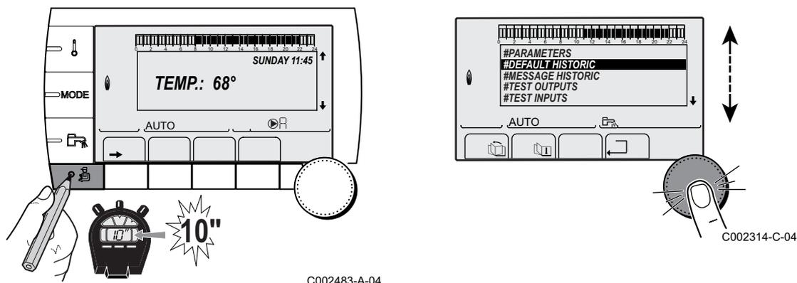
Access: Key → then for 5 seconds or: key, for 10 seconds.
