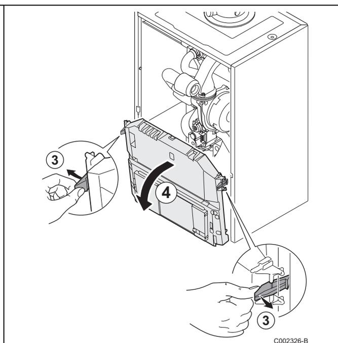
3. Open the holding clips located on the sides
