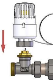
Installation of the thermostatic head for fixed point :
