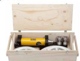
**REMS Python Set.** Oil-hydraulic pipe bender for dimensionally accurate bending of pipes up to 90°. Steel pipes EN 10255 Ø %–2", multilayer composite tubes Ø 32–75 mm. Drive unit with back former supports, upper back former support with laterally adjustable back former support bearing plate, 2 back formers, bending formers St or V. In sturdy carrying case.
