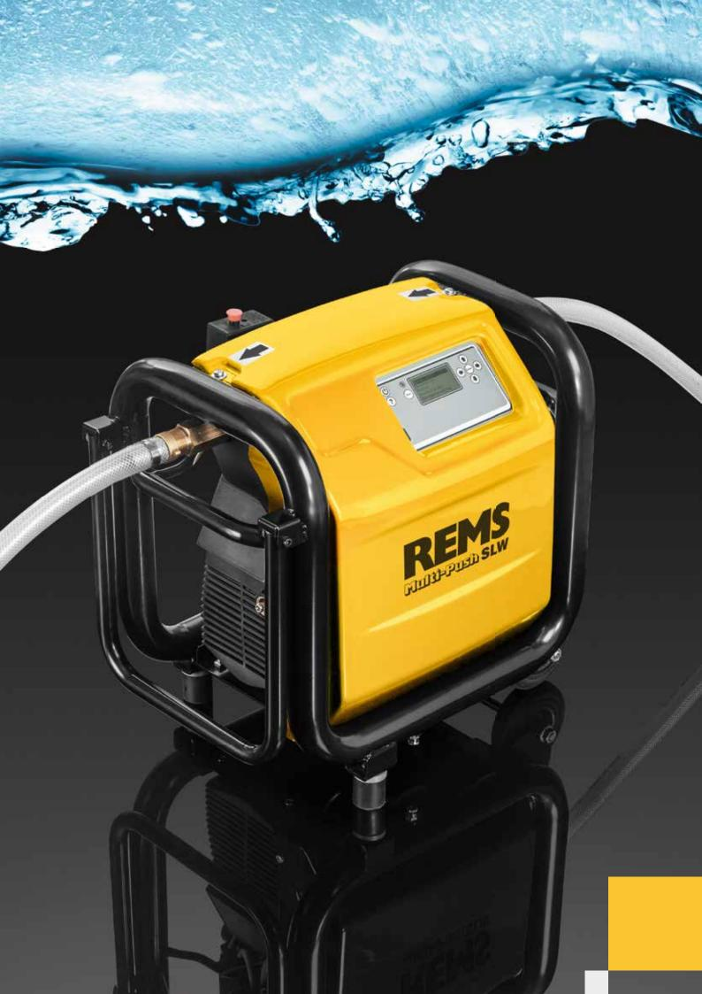
Powerful, compact, electronic flushing and pressure testing unit with oil-free compressor. For flushing with water or a water/air mixture, disinfection, cleaning, preservation of pipe systems, for pressure testing of pipe systems and vessels with compressed air or water, as a pneumatic pump for controlled filling of all types of vessels with compressed air and for operation of pneumatic tools.
