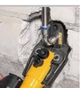
REMS pressing rings 45° (PR-2B) Patent EP 2 774 725
