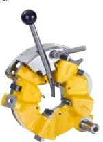
**REMS roll grooving attachment**Robust, compact roll grooving attachment with oil hydraulic in-feed for pipe grooving of grooved coupling systems DN 25–300, 1–12" (page 48).
