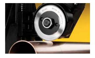
REMS cutter wheels complement the special demands of the various materials. In particular the special hardening process determines the durability of the REMS cutter wheels.
