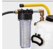
REMS Solar-Push K 60. Electric filling and flushing unit for fast, easy filling, flushing and venting of closed systems. Transport volume ≤ 36 l/min, tank volume 30 l. With centrifugal pump, temperature-resistant for continuous load ≤ 60°C. Transport pressure ≤ 0,55 MPa/5,5 bar/80 psi. Condenser motor 230 V, 50 Hz, 860 W. 2 pieces flexible, transparent PVC fabric hoses ½" T60, each 3 m long, temperature-resistant ≤ 60°C. On sturdy tubular steel frame with air-filled wheels. In box.
