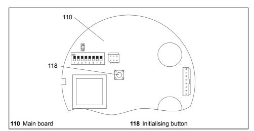
diagram 21 Initialising the path measuring system
