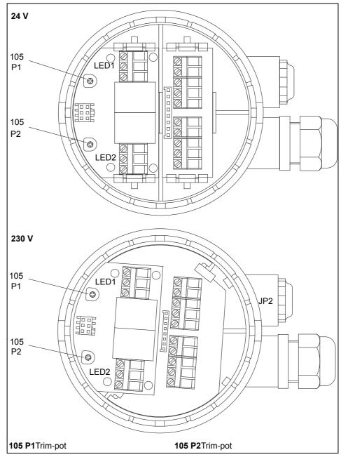
diagram 20 Position switch PCB in cover
