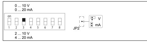
diagram 17 Setting the input signal
