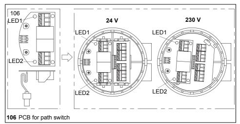
diagram 3 Position switch PCB in cover
