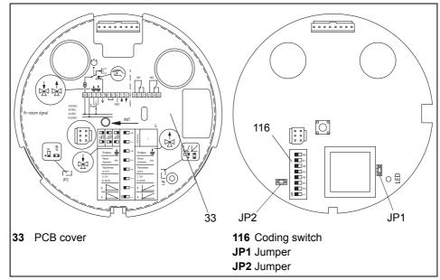
diagram 16 PCB cover, encoding switch and jumper
