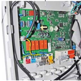
Connection of the first circuit with mixing valve
