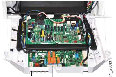
Electricity supply connection for the MIT-IN-2 module
