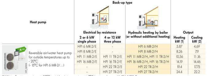
(1) Water flow temperature:  $+35^{\circ}$ C, outside air temperature:  $+7^{\circ}$ C in accordance with EN 14511-2. (2) Water flow temperature:  $+35^{\circ}$ C in accordance with EN 14511-2.
