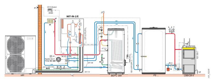
Cascade with an HPI heat pump (with MIT-IN-2 iSystem/E module) and an MCA wall-hung condensing boiler
