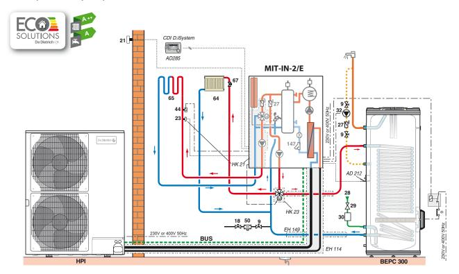
HPI EVOLUTION heat pump with indoor MIT-IN-2 iSystem/E module
