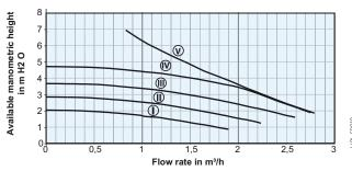
MIT-IN-2 6 and 8: speed-controlled pump I MIT-IN-2 11: speed-controlled pump II
