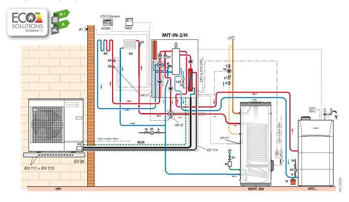
HPI EVOLUTION heat pump with indoor MIT-IN-2 iSystem/H module
