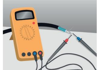
3. Check the insulation resistance of the heating cables. The measured value shall be no less than 50 MΩ.
