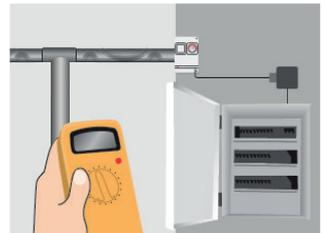
9. Re-check the insulation resistance. Connect cables to connection boxes and to the switch board.
