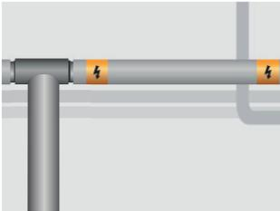
10. After insulation, place safety marking tape on the insulation jacket or pipe trenches for every 5 m. In subsurface installations, a cover ribbon with a warning sign must be laid 10 cm above the cables.
