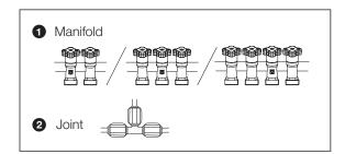
The main advantage of point to point plumbing compared to traditional type of plumbing is the possibility of reducing the number of joints. That way you can decrease the potential risk of leakage.
