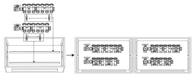
Pipes are screwed onto HERZ Drinking water manifolds. The pipes have to be correctly aligned, so the manifold is not loaded with a bending moment. When using copper or plastic pipes take into account pressure and temperature limits of the selected material. When assembling, use a suitable assembly tool that adapts to manifolds end connections. We recommend you to use HERZ Pipefix G3/4" connection.
