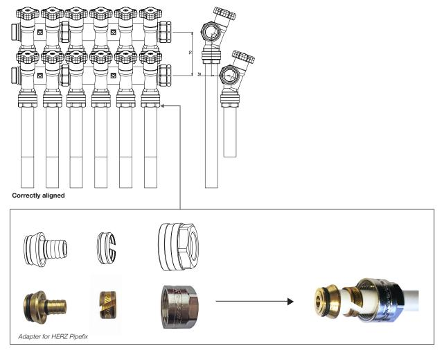
Following assembly, the connections of the manifold must be checked for water-tightness by the installer. All engineering standards and recognized regulations must be adhered to by these specialist staff. If there are impurities in the medium (water too hard, dust, etc.) there should be a filter installed, in other case the impurities can damage the seals of the valves inside the manifold.
