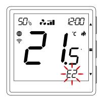
E2 - Break in the external temperature sensor circuit
