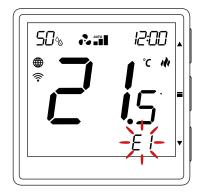
E1 - Short circuit in the external temperature sensor circuit
