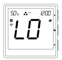
LO - Temperature measured by the internal sensor too low
