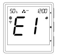
E1 - Short circuit in the internal temperature sensor circuit
