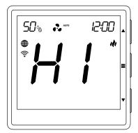
HI - Too high temperature measured by the internal sensor
