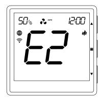
E2 - Break in the internal temperature sensor circuit
