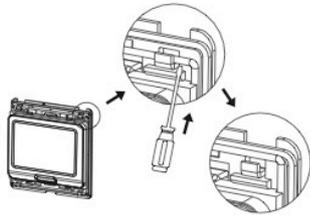
③ Mounted the backing plate in the wall socket by screwdriver.
