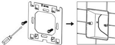
④ After connect wires (see right diagram), the thermostat mounted on the backing plate and remounted the cover and frame.
