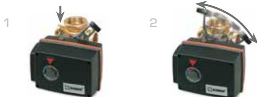
1 To operate the valve manually, push the button and use the lever. The electric current is automatically disconnected as long as the button is in the lower position.
