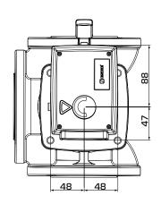
Installation dimensions for Actuator Series 90 with ESBE series MG, G, F, T/TM, H/HG and BIV mixing valves
