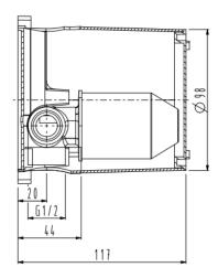
UH00367; inlet 2 X 1/2", outlet 1 X 1/2", recessed armature fitted with mixer head 35 mm diameter
