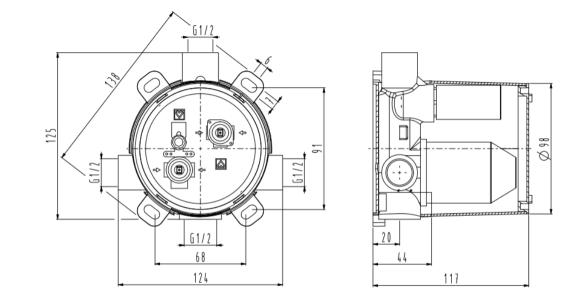
UH00368; inlet 2 X 1/2", outlet 1 X 1/2", 1 X 3/4" recessed armature fitted with mixer head 35 mm
