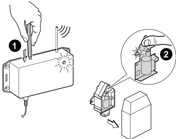
Each outside temperature sensor is given a unique identifying number in the factory, which enables the radio module to recognise it. This identifying number is transmitted to the radio module by the pairing sequence described below.
