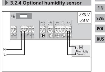
Humidity sensors (to be provided by the customer) serve for dewing protection in the cooling mode.
