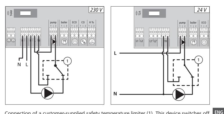
Connection of a customer-supplied safety temperature limiter (1). This device switches off the pump and sets the input to TL if too high flow temperatures for the floor heating are detected. If the TL input is switched, the base station shuts down all actuators automatically.
