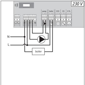
The boiler connection allows the control of a heat generator. Additionally, a pump can be controlled directly.
