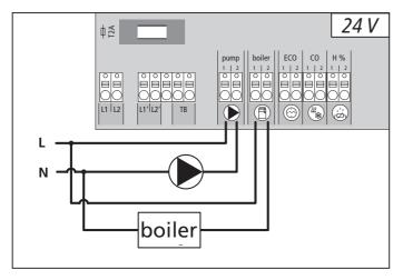
The boiler connection allows the control of a heat generator. Additionally, a pump can be supplied and controlled directly.
