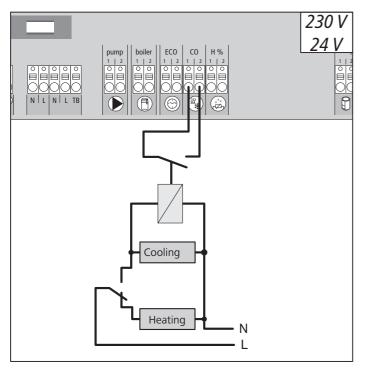
If an external change-over signal is used, the overall installation switches accordingly between heating and cooling.
