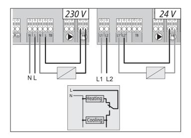
If no external change-over signal is available, the internal pilot function of the base station can be used for switching the overall installation between the operating modes Heating and Cooling. A relay used by the base station for switching over is used for this.
