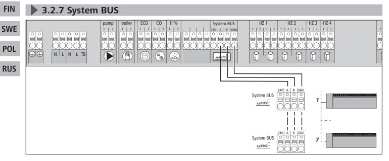
A maximum of seven base stations can be interconnected via the system BUS (syBUS) in order to exchange global system parameters. After completing the wiring, the base stations must be paired – see section 4.2 For a line diameter <6 mm, a strain relief must be provided by the customer.
