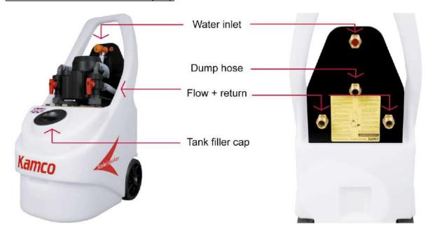
**Flow and Return Hoses:** need to be connected to the equipment being descaled so that a circuit is created allowing water to travel back to the Scalebreaker pump.
