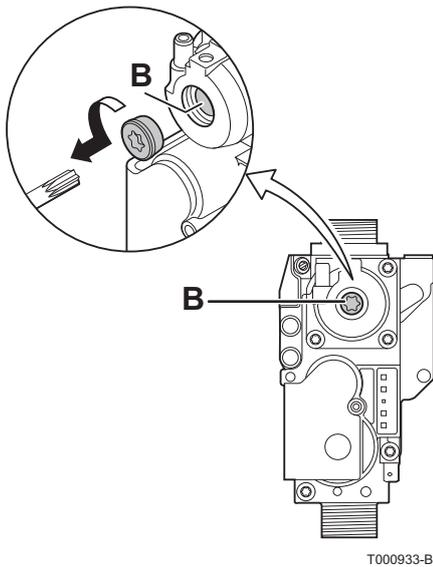
6. If this rate does not match the required value, correct the gas/air ratio using the adjustment screw B on the gas valve unit.
