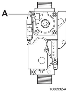
7. If this rate does not match the required value, correct the gas/air ratio using the adjustment screw **A** on the gas valve unit.
