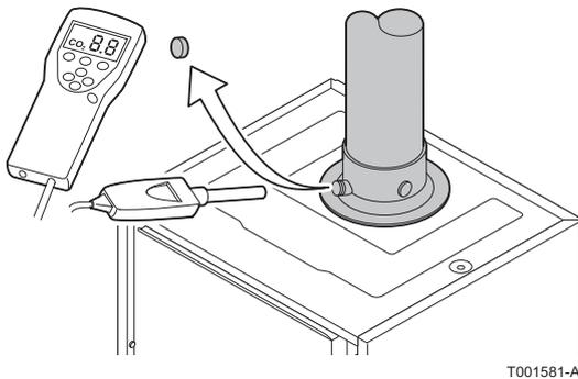
1. Unscrew the plug of the flue gas measurement point.
