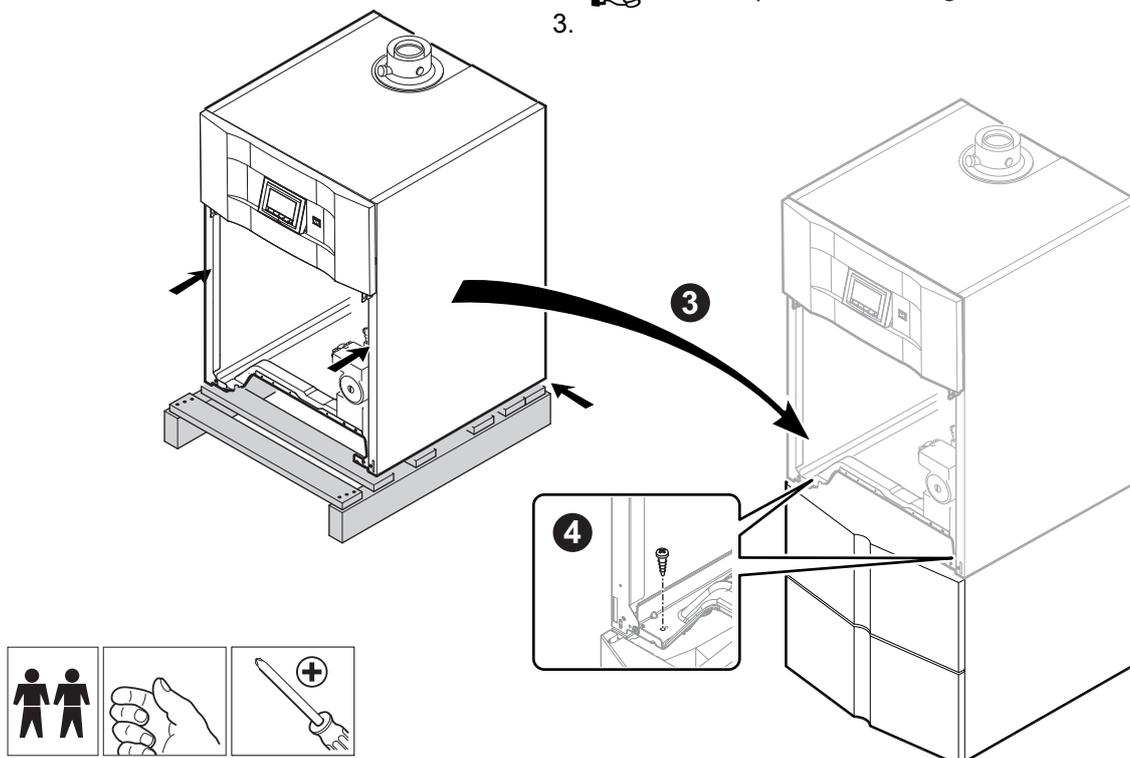
Position the boiler on the DHW tank.
