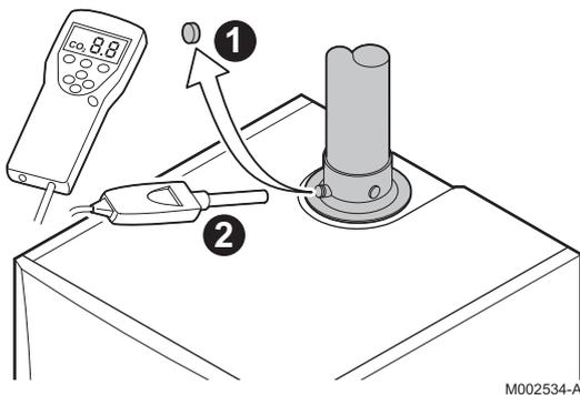
The check on combustion is done by measuring the percentage of O<sub>2</sub>/CO<sub>2</sub> in the flue gas discharge flue. To do this, proceed as follows:
