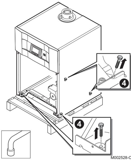
5. Lift the boiler and position it on the ground
