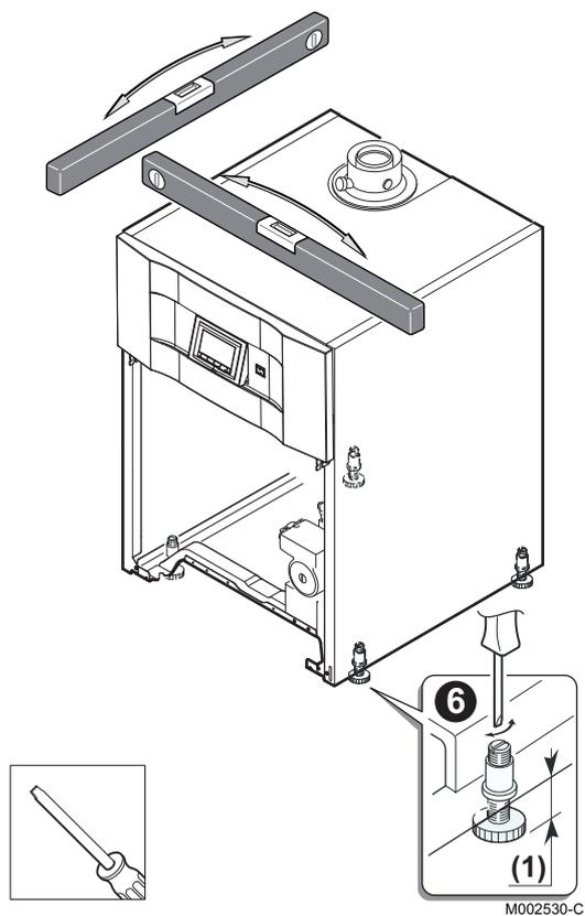
6. Level the appliance using the adjustable feet.
