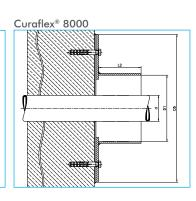
Curaflex® pipe sleeve 8000/T split version. For installations with existing pipeline in the wall
