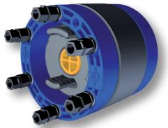
Curaflex Nova® gasket inserts fit many different diameters. The sealing insert is adapted to the pipe / cable to be sealed by removing the rubber modules (DDE). The modules to be removed are shown in the table below:
